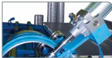
Automatic Corrugation Unit
