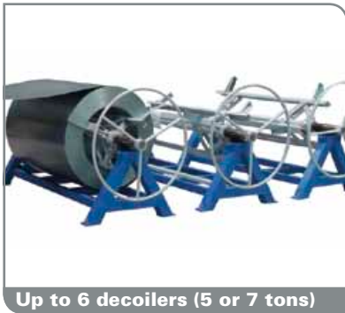
Up to 6 decoilers (5 or 7 tons)
